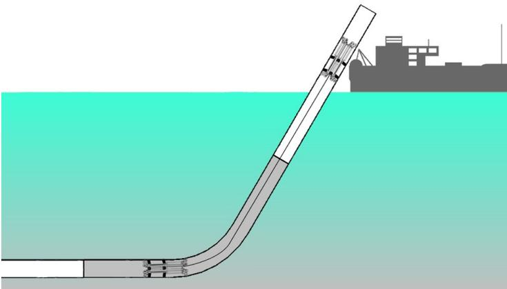
Fig. 8 Both DPT crawlers advance and the bottom crawler inspects the newly laid section
