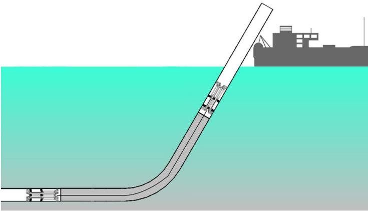
Fig. 7 A new length of pipe has been welded, the barge advanced and a new pipe section has been laid on the sea bottom.
