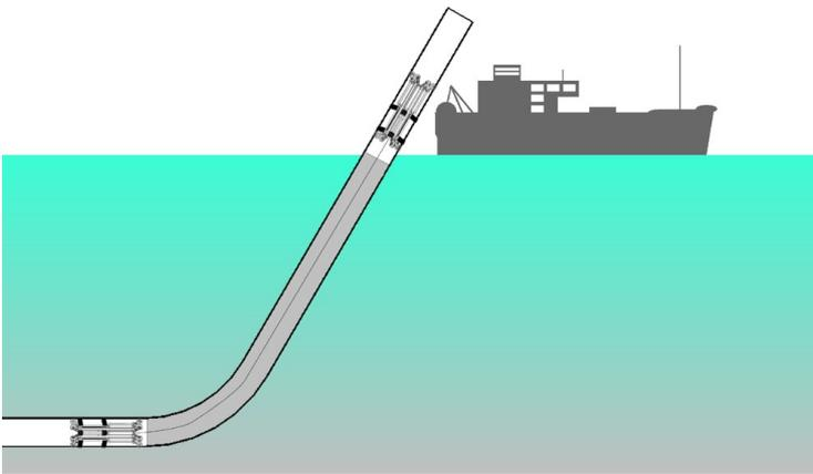
Fig. 6 General layout showing two DPT tractors inside a submarine pipeline being laid from a barge
