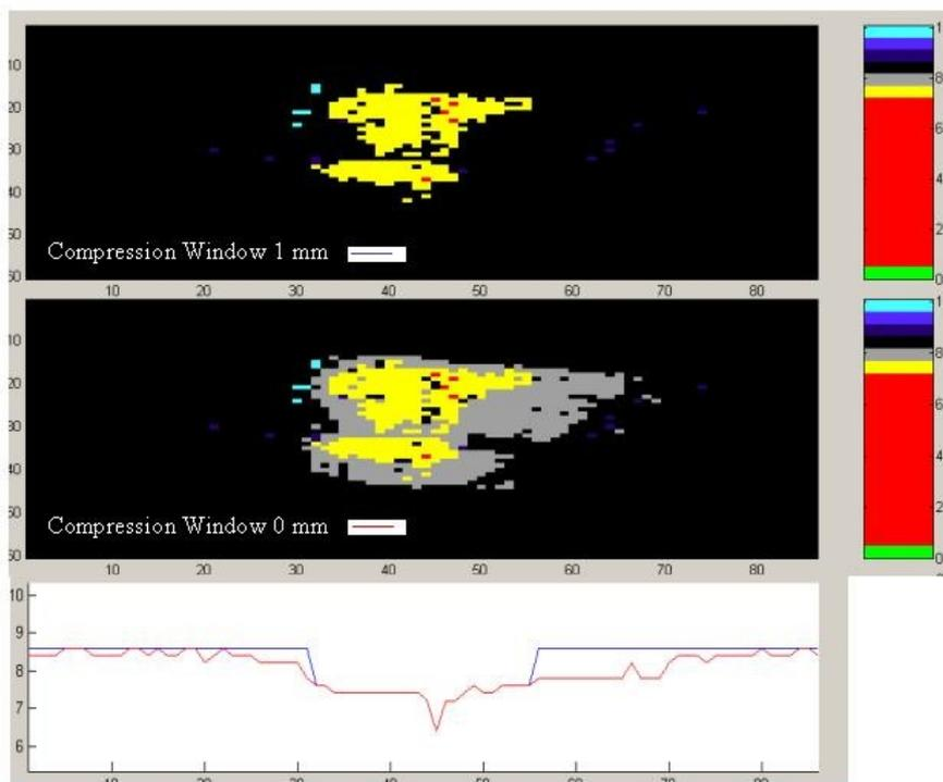
**Figure 3: The compression window will affect how shallow deviation from the nominal wall thickness will be stored in the data.**
