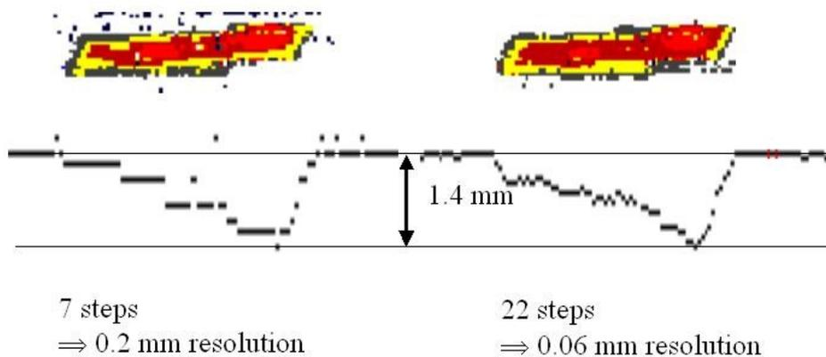
**Figure 2: Depiction of a metal loss defect measured with different resolution.**
