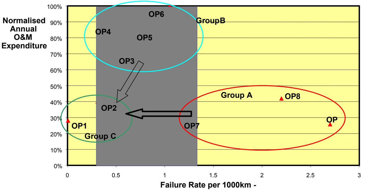
Figure 4 : Assessment of O&M expenditure versus pipeline risk (failure rate)
