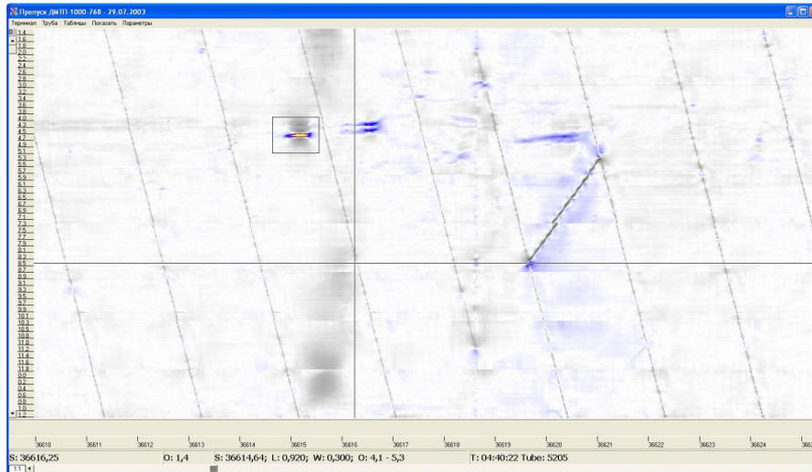
Here is TFI inspection plot that shows a pipe layout. Nearly all defects here are of metallurgic origin. Defects of longitudinal weld seam and girth weld defects are well detectable, using joint MFL + TFI technology.
