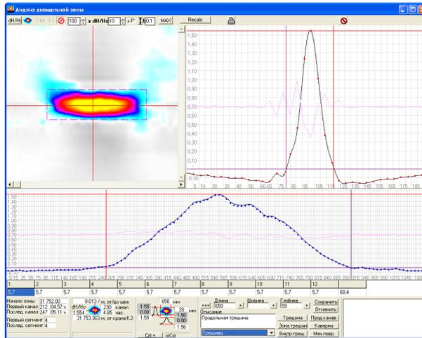
Now the problem of discrimination in identification of mid-wall laminations and SCC cracks is solved. Statistically, nearly 95% of such mid-wall laminations are opened in the inner pipe wall, only insignificant number of such cracks being opened in the outer pipe wall. The longitudinal crack is clearly seen on the colored TFI inspection plot.
