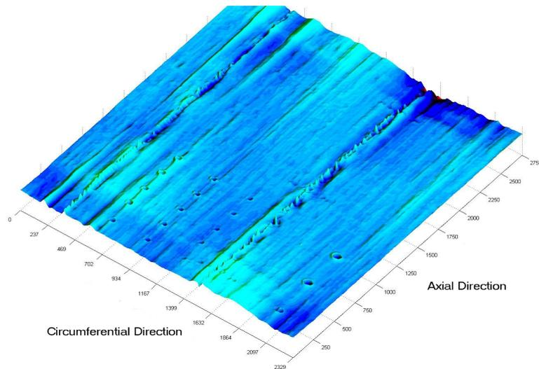
Research work of second trend, i.e. measuring signals initiated by defects in different fields is practically completed. There were opinions of scientists from other countries that it is impossible to detect small stress corrosion cracks with minor opening, using only magnetic method. Our specialists also made conclusion that zones of minor SCC cracks are detected by MFL tool only because local stress state of pipe metal body arises above such zone, which is detected by MFL tool.
