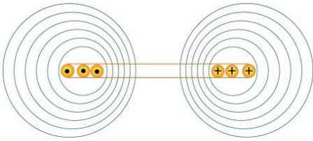
Figure 1. Magnetic Field created by a coil in air
