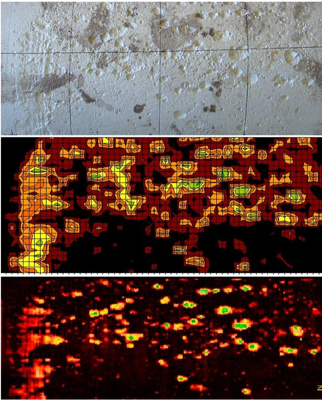
Figure 6. Corrosion, Conformable Array Scan, LASER Scan
