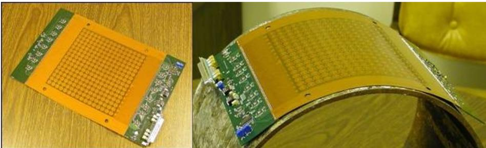
Figure 5. Conformable EC Array
