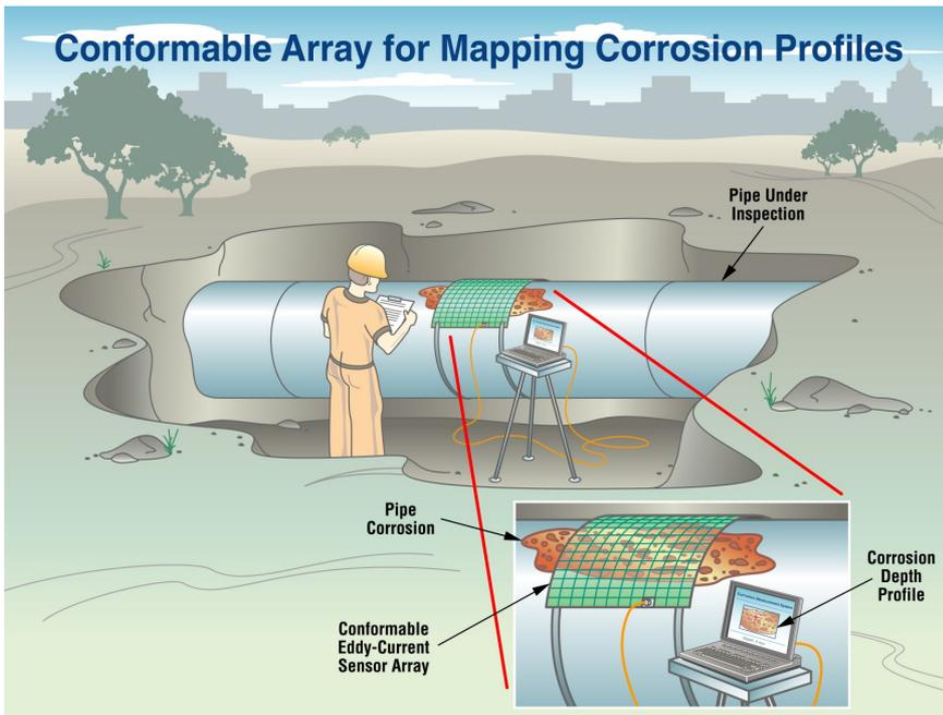
Figure 4. Flexible array concept
