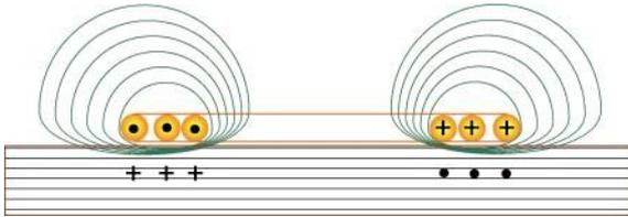
Figure 2. Magnetic field created by eddy current coil near a metallic surface
