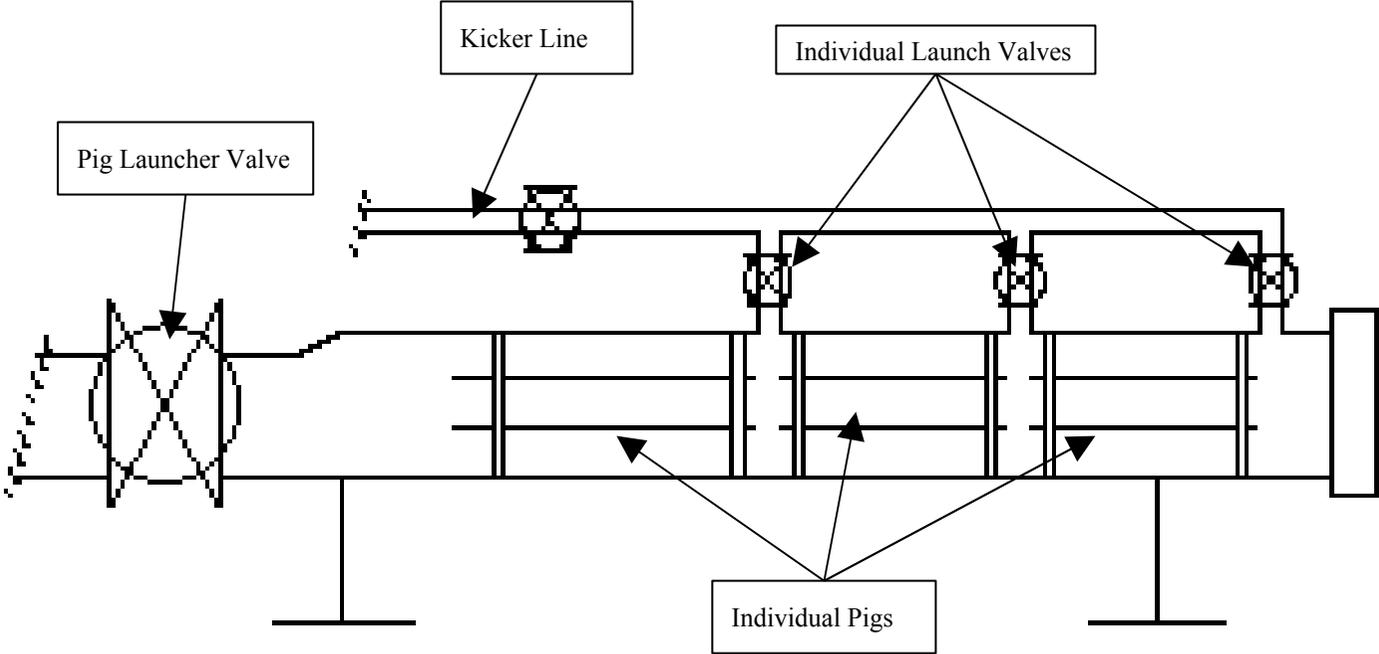
**Figure 2. Vertical Multiple Pig Launcher**
