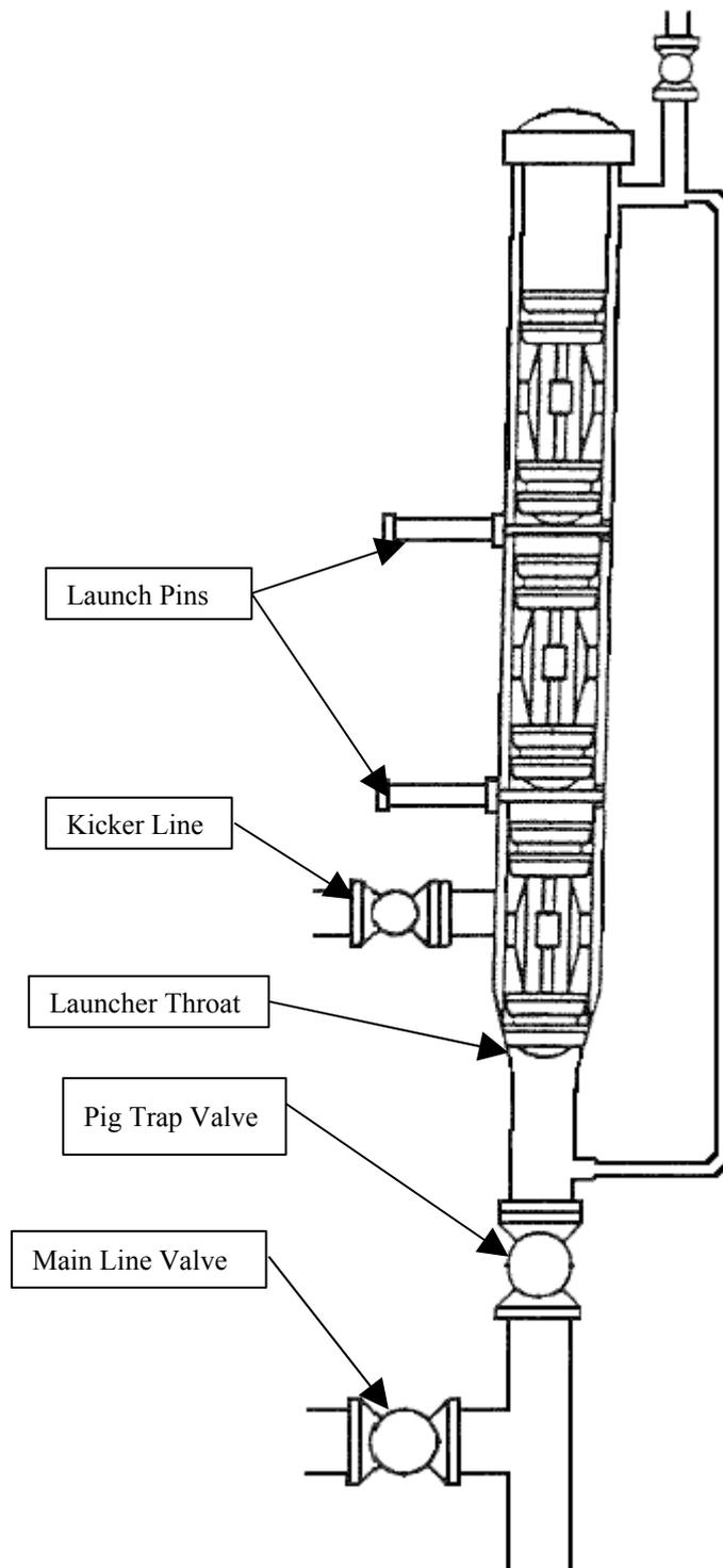
Figure 3. Automatic Sphere Launcher
