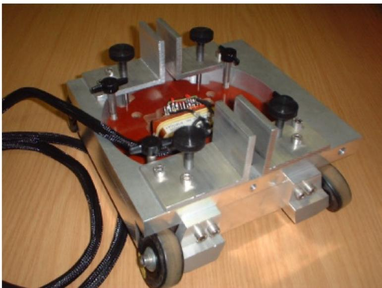
**Figure 5 - Probe Support Trolley**
