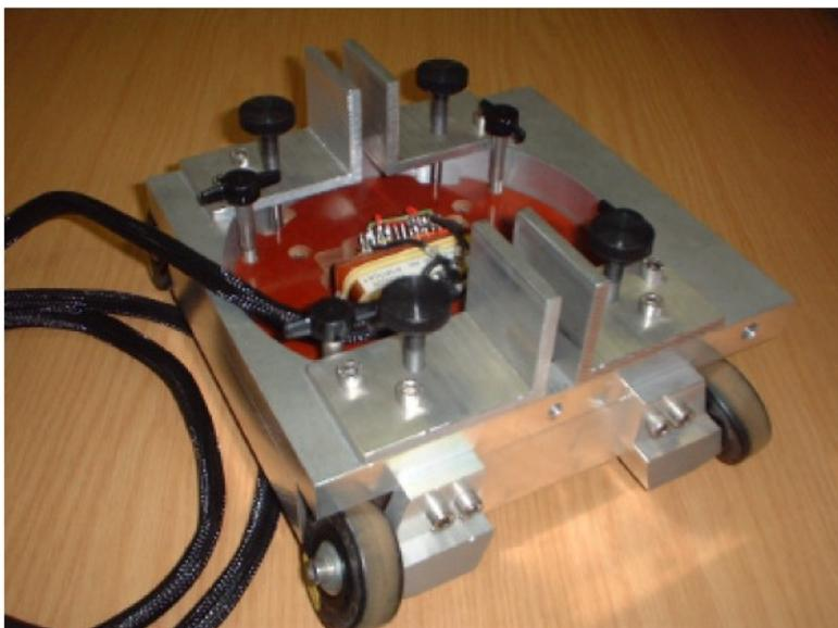
**Figure 5 - Probe Support Trolley**
