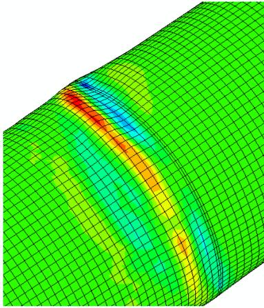
Figure 5 - Plastic Strain Contour Plot of a buckle at outer surface
