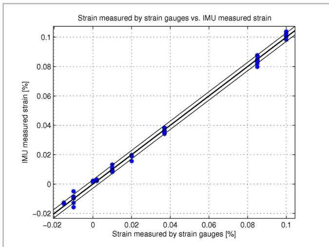
Figure 7: Strain gauge readings plotted against IMU strain results
