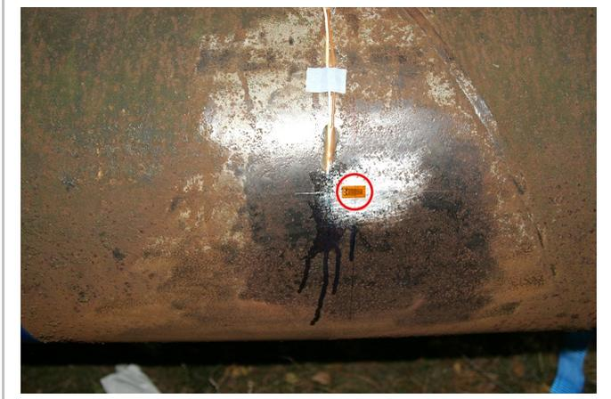
Figure 4: Integrated strain gauge (red circle) for external strain measurements
