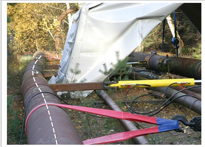
*Figure 1: 4-point bending with hydraulic jacks*
