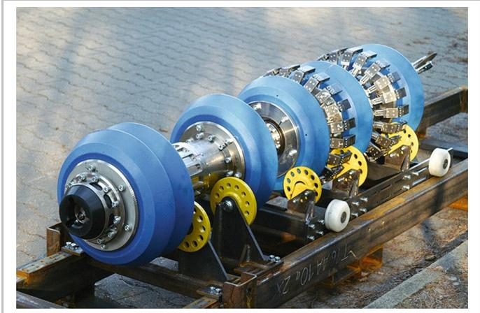
Figure 3: 16" RoGeo·Xt with XYZ mapping and HiRes ID mapping module
