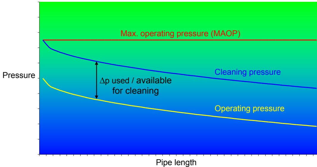
Usually the differential pressure required for cleaning depends on the deposit characteristics. In order to minimize additional power requirements a cleaning head will be chosen that only generates the power necessary to remove a particular deposit. The cleaning power applied is the product of the flow rate through the pig and the pressure difference over the pig.
