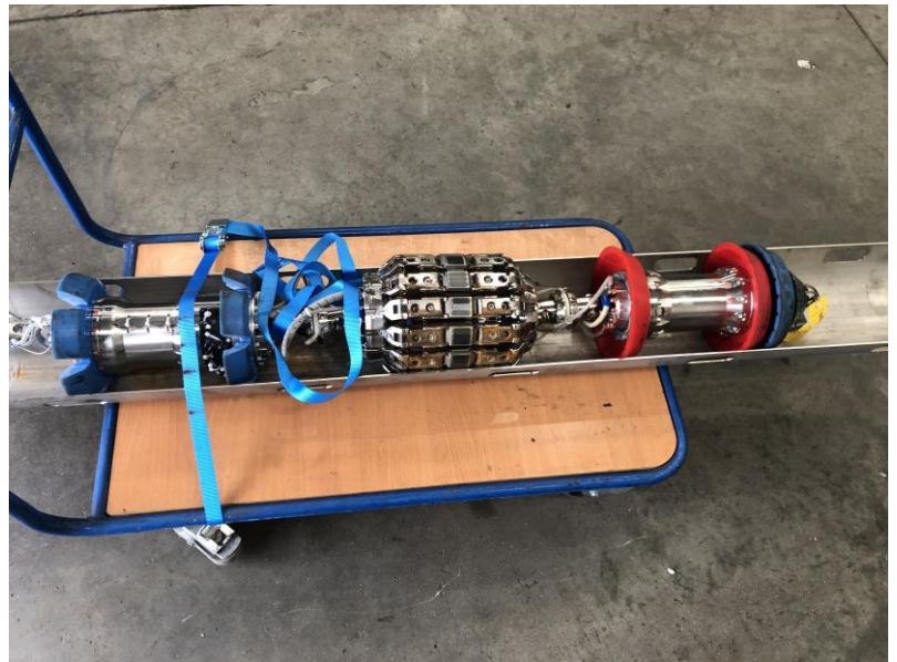
Figure 4: 8" ROSEN MFL inspection tool tracked during the operation
